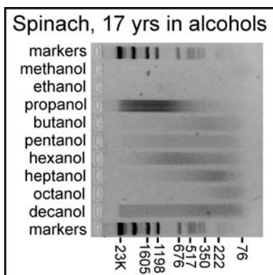
Fig. 1. Gel of spinach DNA stored 17 yrs. in various alcohols.
